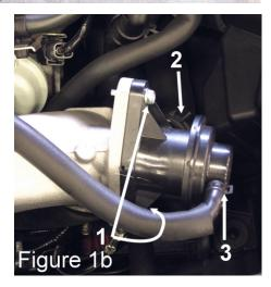
Replace the two factory bolts, recirc and vacuum hoses and clamps.
